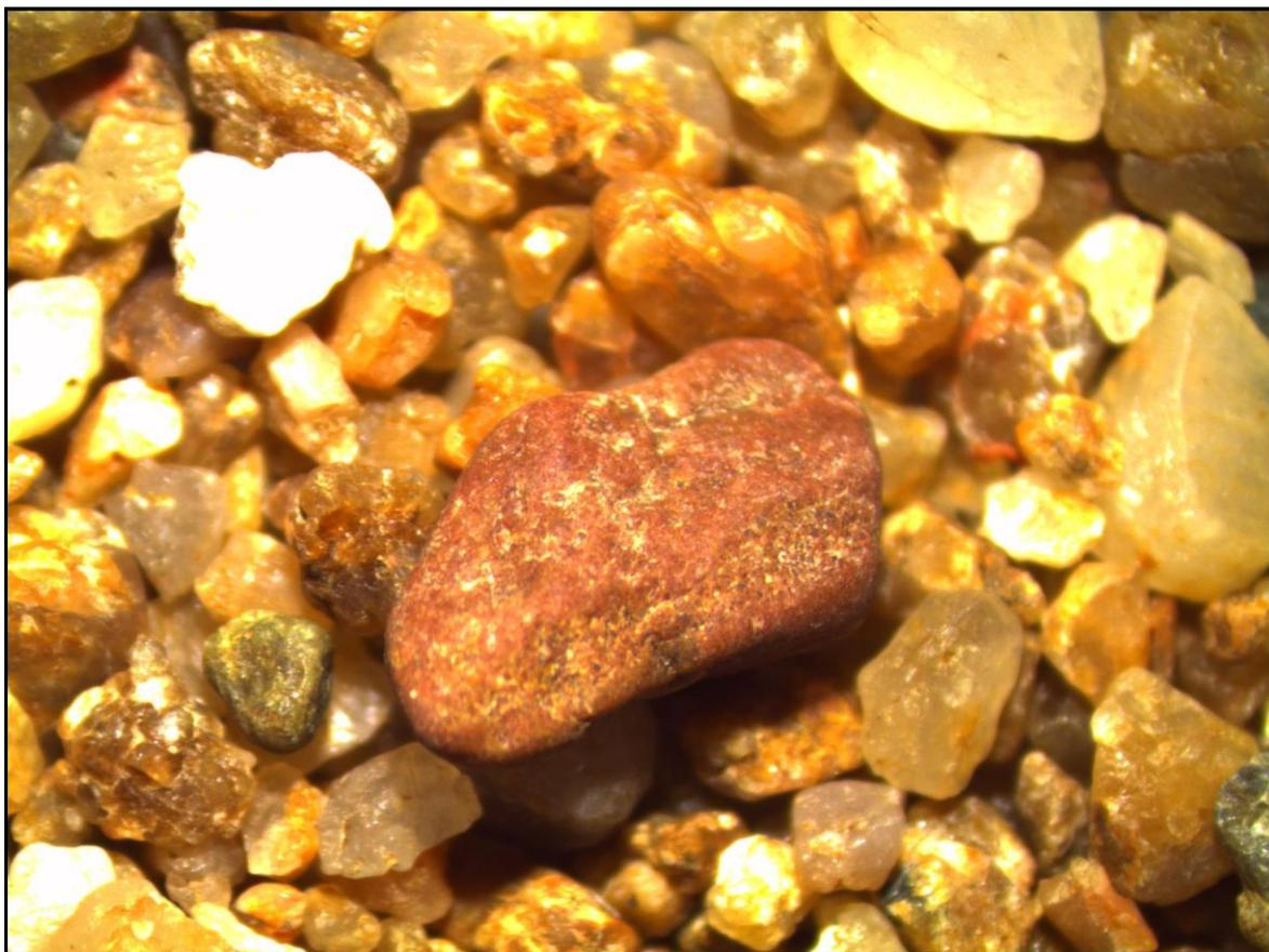
**Figure 3:** Image of the coarse fraction composed of granite and quartz
