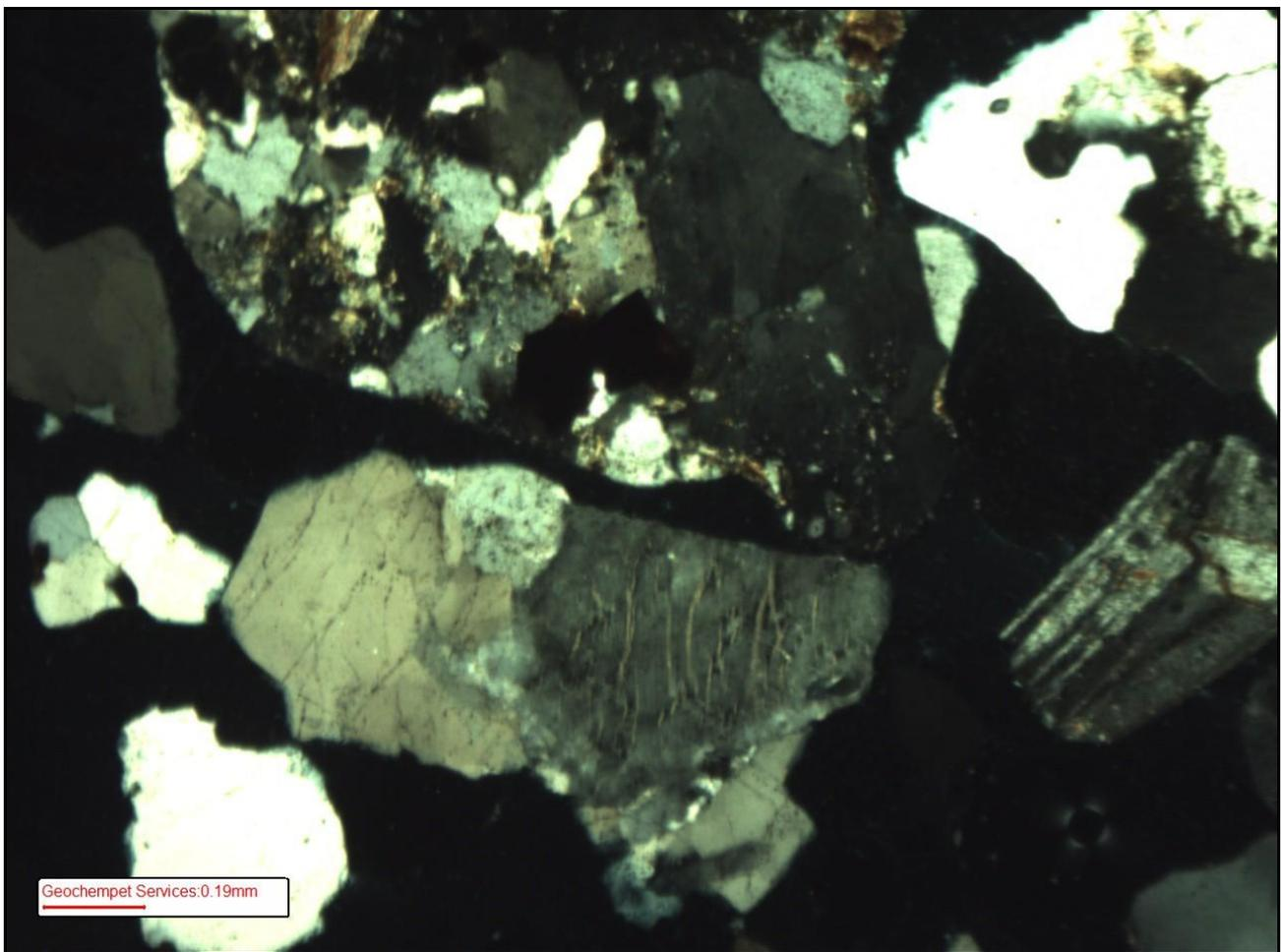
**Figure 4:** Photo-micrograph taken at low magnification with transmitted cross polarised light. Image shows the typical mineral assemblage observed throughout the slide with a mixture of free grains of feldspar and quartz as well as lithic clasts of granite.
