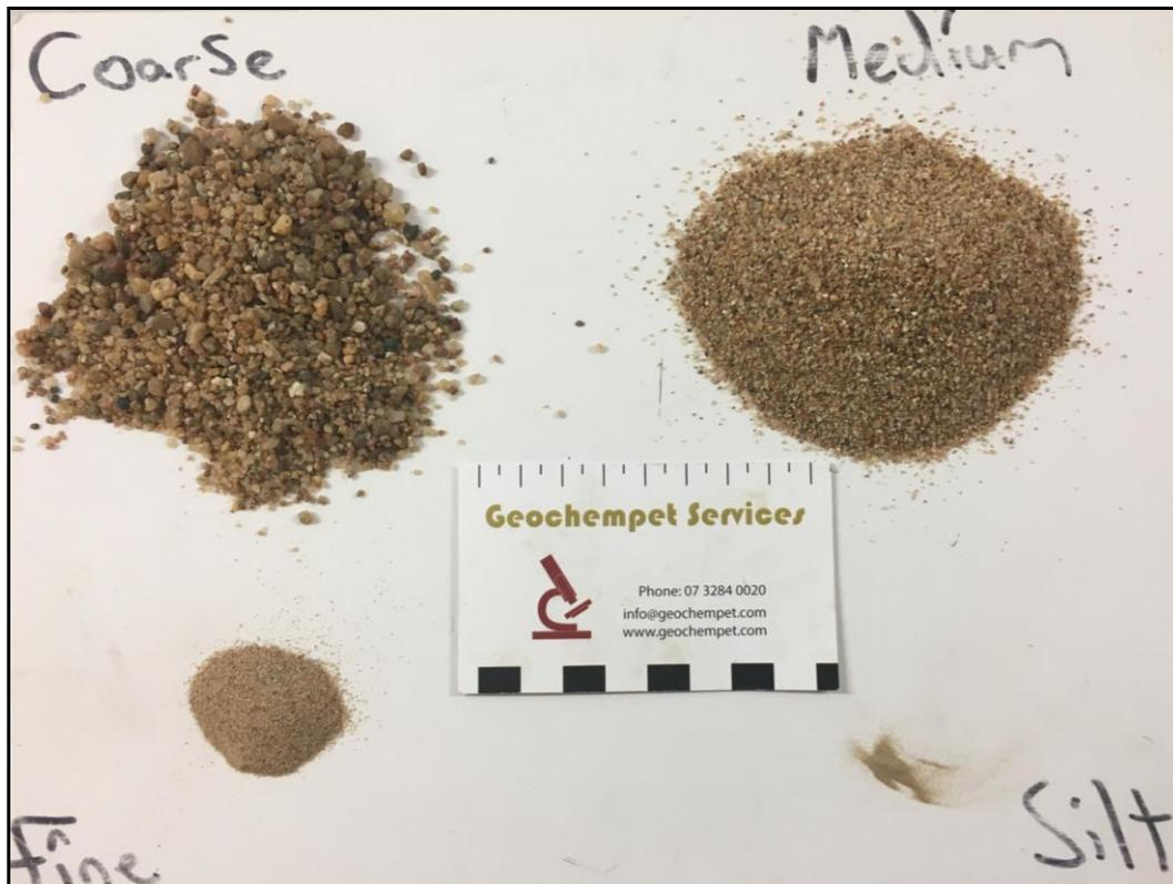
**Figure 2:** Digital image of sieve fraction as recorded above.
